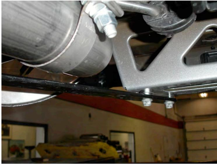
8. Install  $\frac{1}{4}$ " thick stainless steel spacers (SPCR\_CA10\_1), one for each side, between cross brace and bottom of the car and tighten the (4) 15 mm bolts. (This is the brace that runs directly under the X-pipe). Tighten and adjust as needed. Make adjustment so that X-pipe is situated above the cross brace by approx  $\frac{1}{2}$ " to  $\frac{3}{4}$ " after tightening. See picture below.
