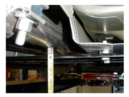
11. For Convertibles only, using (6) 15mm bolts, bolt in the longer cross brace supplied with kit CA11CONVKIT, with cutout toward the front of the car. See picture below:
