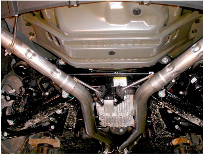
6. Install 3" hanger clamps and muffler outlets using sealant.
