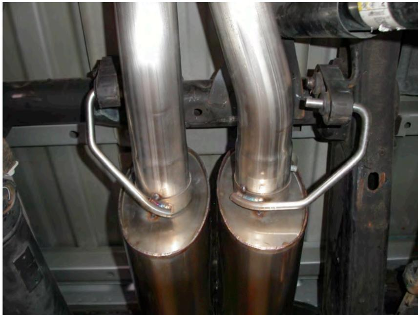
9. Install tail hanger using (2) 3" clamps.
