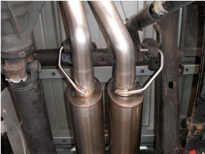
9. Install Right and Left tail hangers to factory bolts in trailer hitch using farthest ones forward 14mm, (see picture).
