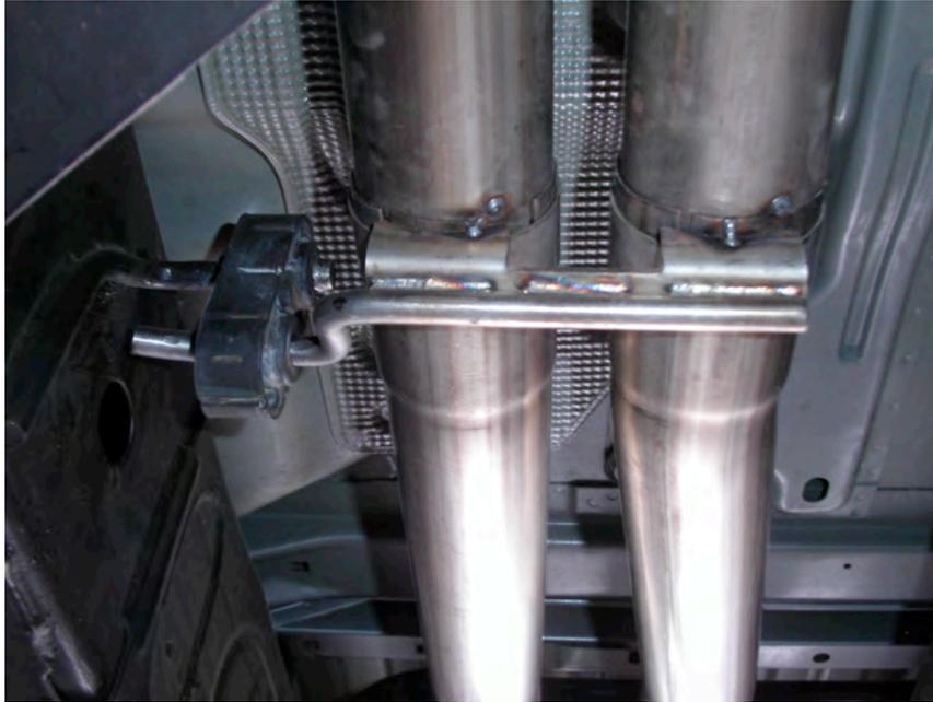
7. Install mufflers using (2) 3" clamps.
