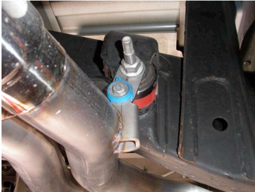
9. Install tail pipes and tips using (2) 3" clamps and grommet with 3/8" bolt, washers and nut.
