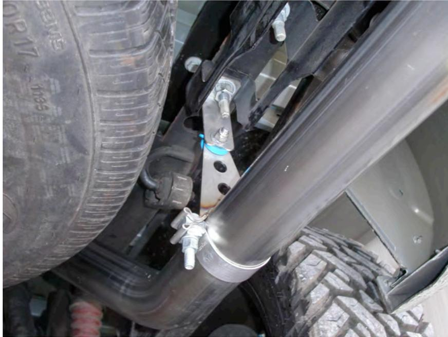
10. Install Right and Left tail pipes and 3" clamp hangers with grommets and 3/8" bolts and nuts.
