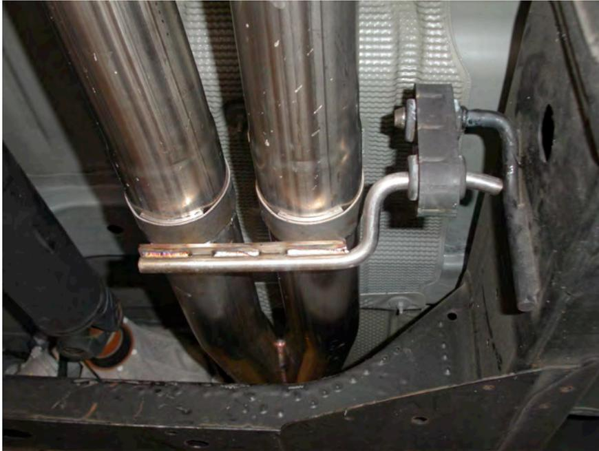
7. Install mufflers using (2) 3" clamps.
