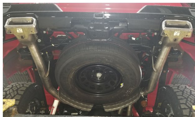
Detail 13: Rear tails and hanger brackets installed.
