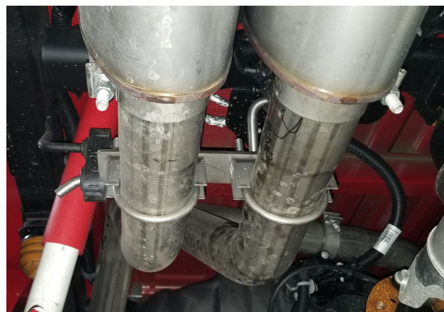
Detail 12: Tail hanger assembly
