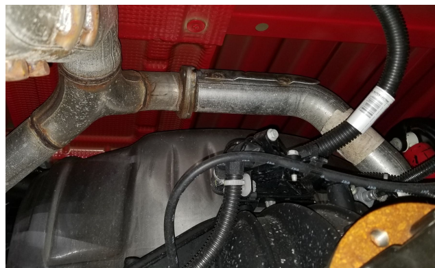
Detail 4: Left tail OEM flange connection
